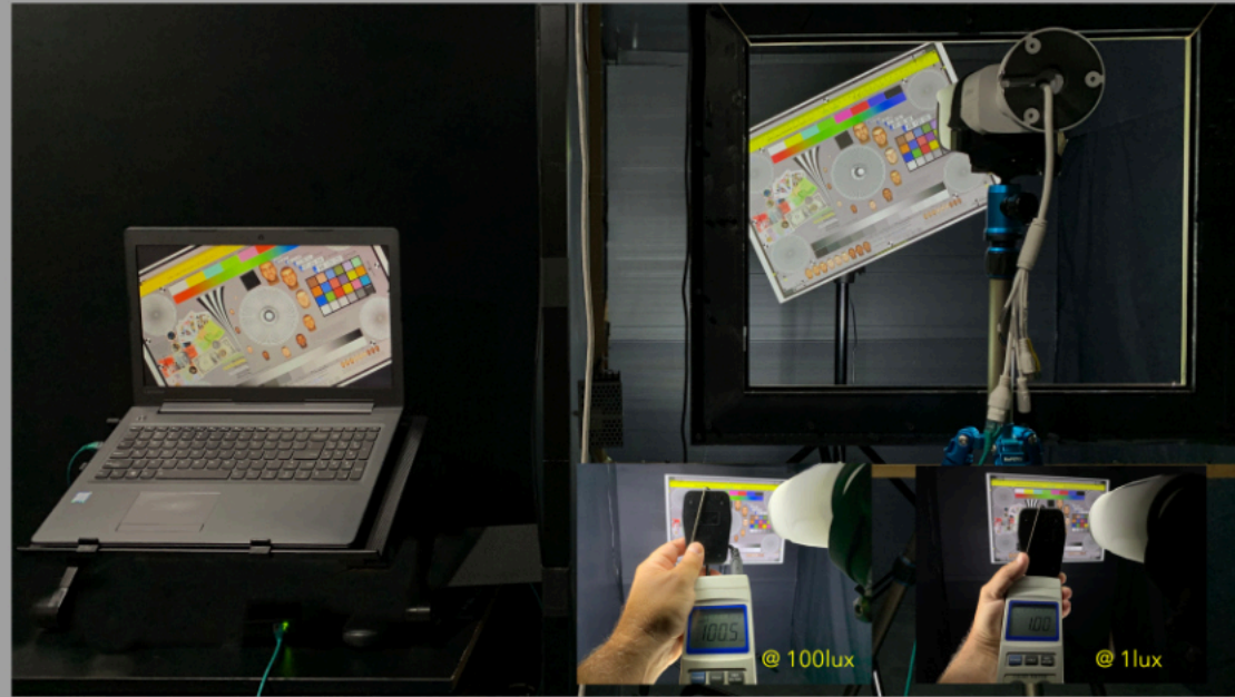
Our ViDi Labs A3 v5.2 chart test jig, mounted on a stepper motor axis, with variable rotating speed By varying the revolution speed (rev/s) and light levels we can simulate almost any condition in order to test camera quality at various settings
