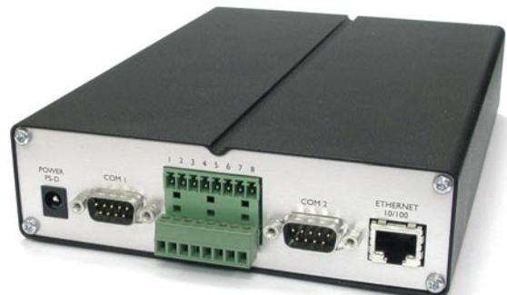
On the back panel we have the serial ports, alarm input/output terminal, RJ-45 LAN port and power supply socket.
