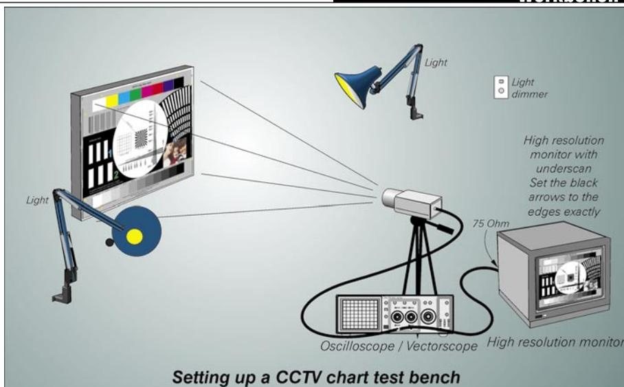
can also test the camera's minimum illumination. Naturally, if this needs to be tested, this whole operation would need to be conducted in a room without any additional light. Also, if you want to check the low light level performance of your camera you would need to obtain a precise lux-meter.
