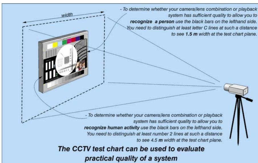
as to see 1.5 m width, use the same formula mentioned earlier. This test can be very useful to find out if your camera/lens combination gives sufficient details. Such measurement is even more informative in determining the playback quality of a digital video recorder since there is no objective method of determining compression/decompression quality in CCTV.
