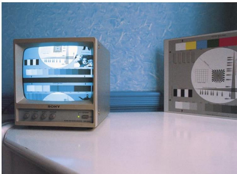
their resolution tested with such a monitor, but the majority of color cameras (which have up to 480 TV lines) should be OK for testing with such a monitor.
