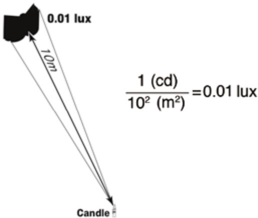
At 10 meter distance the illumination drops to 0.01 lux.
