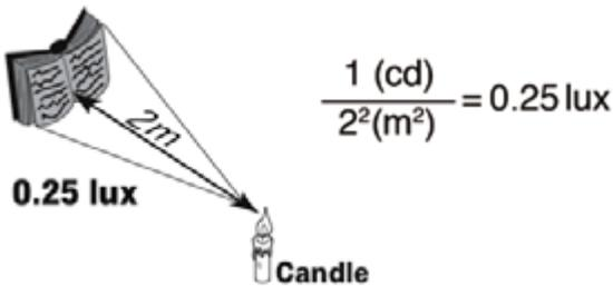
0.25 lux, At 3.16 meter distance the illumination falls to 0.1 lux.
