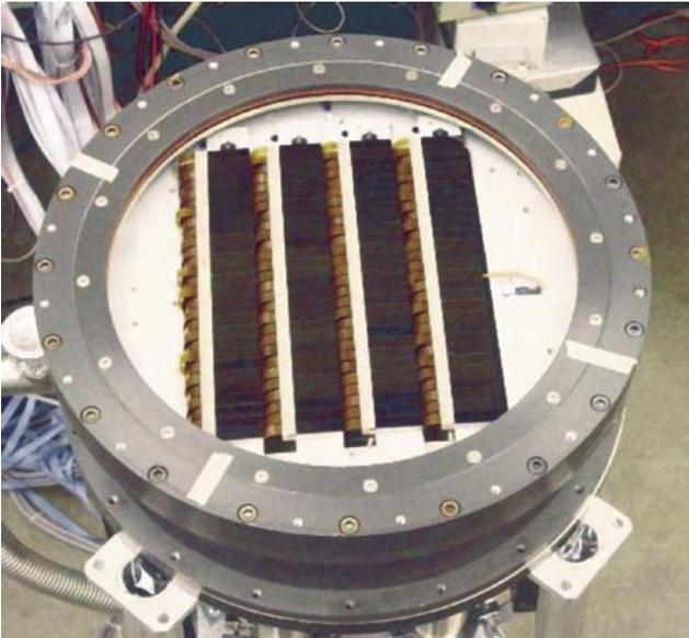
The CCDs are mounted on four separate fingers, 28 CCDs each. Under steppor-motor control, the angles between the fingers can be altered to align the parallel readout direction of the CCDs with the paths of drifting stars. The motor controller is attached to the outside of the telescope.
