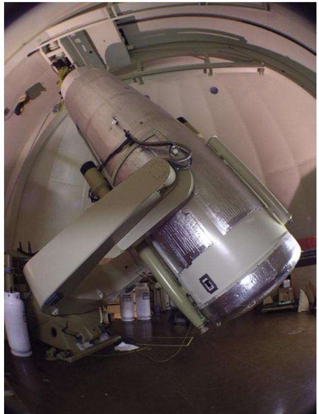
the camera electronics to a controlling computer (quest7). The camera electronics are cooled with chilled water.
