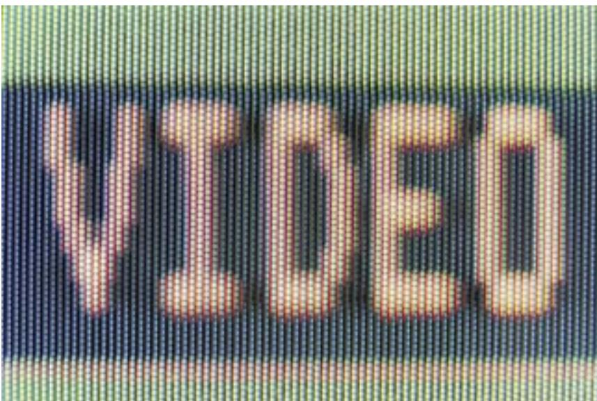
The RGB structure of a CRT monitor screen
