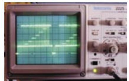
A basic measuring tool in television and CCTV - Oscilloscope. Without it - it is impossible to see the video signal levels and synchronisation pulses. On the photo above, horizontal synchronisation
