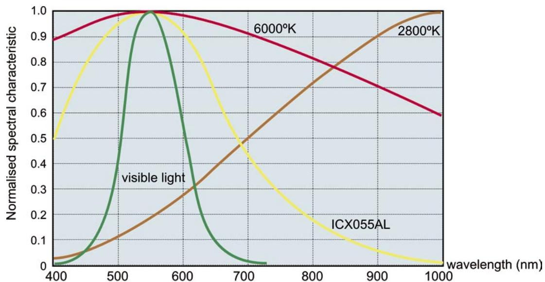
**Fig.2 - Spectral characteristics of the sensor and light sources**
