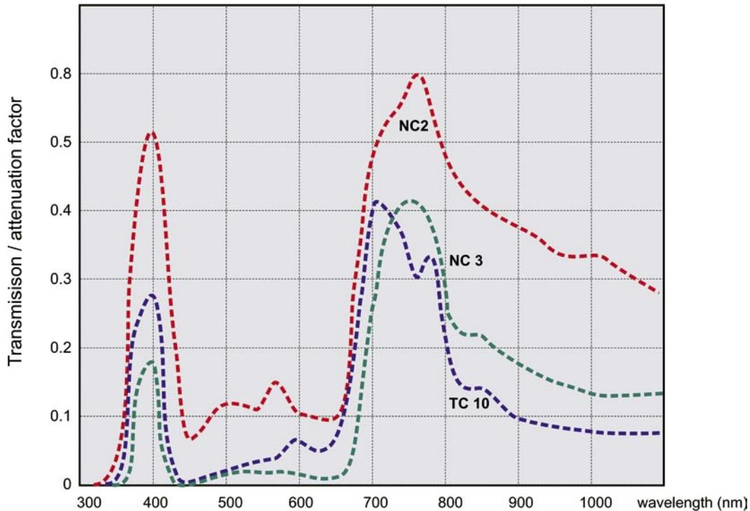
**Fig.3 - Spectral characteristics of ND filters**
