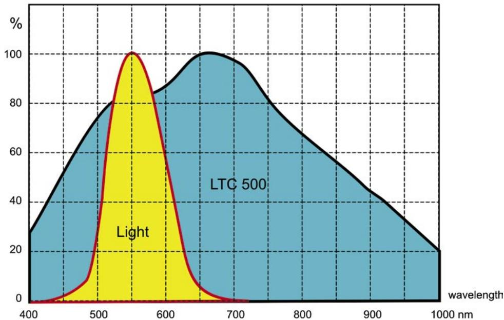
Fig.1 The spectral response of the Philips LTC 500 CCTV camera
