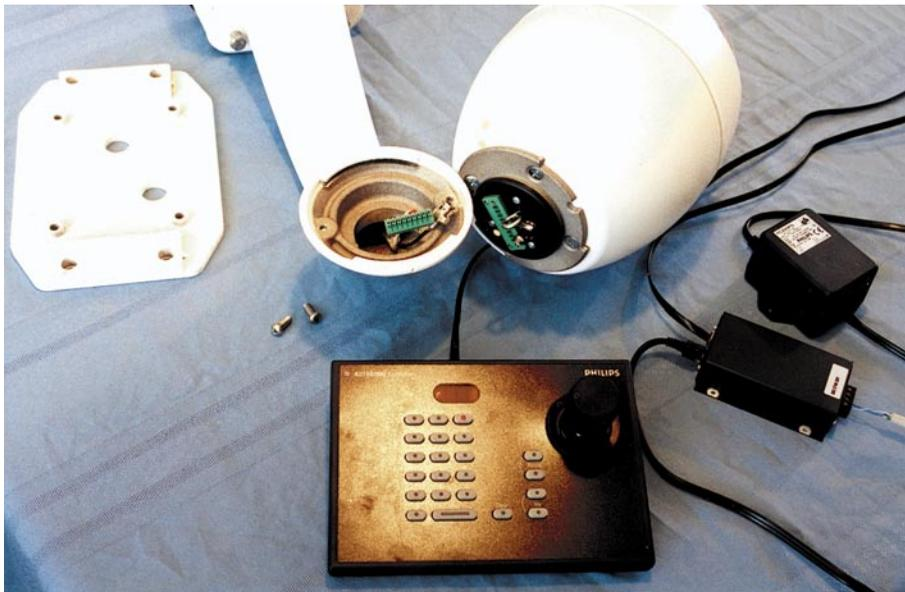
*These are all the components required to set-up the G3 PTZ dome*
