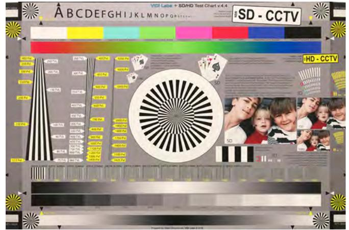
The ViDi Labs test chart in JPEG format (8-bit) = 2.4MB
