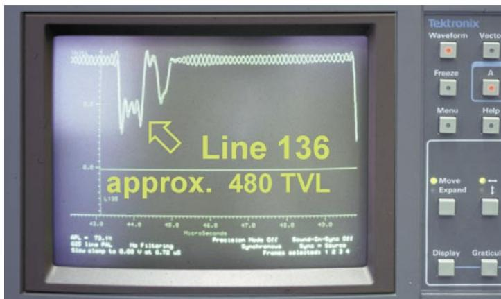
this camera has 480 TV lines. Such a high resolution does offer clear and crisp images, although you need to have a high-resolution monitor to
