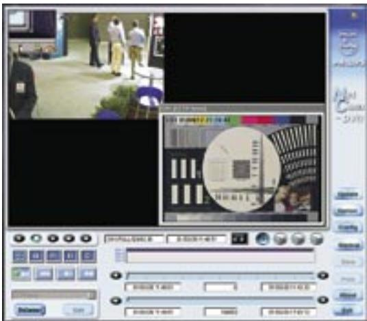
The Net-Cam DVR has a simple and intuitive control window. The play-back (top left hand corner) can be in full screen or quad. The live image (shown here with the CCTV Labs Test Chart) can only be in separate windows floating on top of the control window (up to 4, for all cameras connected to the Net-Cam DVR). The maximum resolution of the live images is limited to CIF size (360X243) in order to save the speed of the compression chip for
