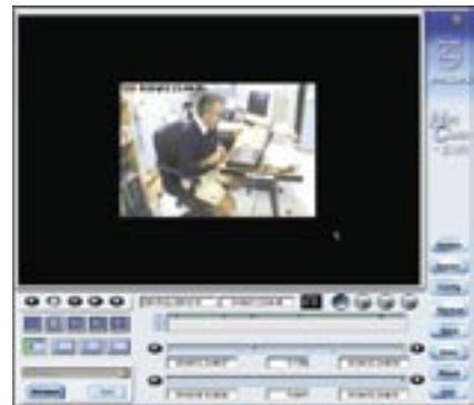
A little "M" on the live and playback image indicates detected movement. Also, the time scale has two colours to indicate normal and movement recording. In addition, during live monitoring via the LAN and when playing back a little red "M" appears at the bottom right hand corner indicating that the camera logic has detected motion. It may not be the most sophisticated VMD in CCTV, but it does work. Of course, sensitivity of the VMD can be adjusted.
