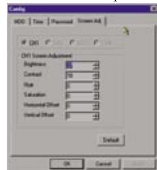
Individual video signal adjustments can be made for all 4 channels
