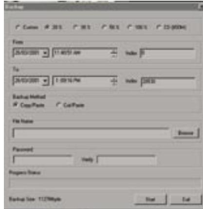
The Net-Cam DVR allows not only to export BMP images, but also backup a sequence of events selected on time basis, or index. You need the Net-Cam software to at the same time.
