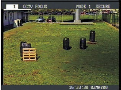
Even a fast moving cloud did not trigger the Axiom VMD
