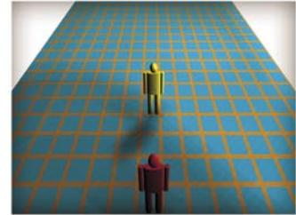
*A two-dimensional plan (above, left) shows that the camera's triangular field-of-view covers the three people satisfactorily, but when we take the rare step of looking at a side elevation (above, centre) the blind spot is revealed. The actual view from the proposed camera is generated by the computer (above, right) so that even non-technical contributors can comment on its suitability.*
