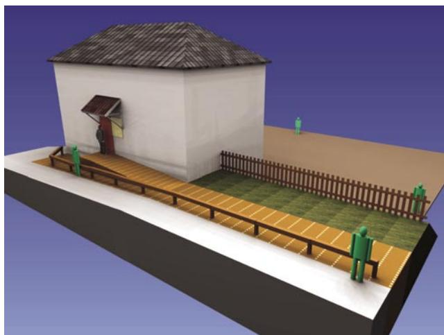
*Survey measurements took less than 1 hour in order to create this site as a 3D computer model. The green figures are 1.6m human-sized 'markers' placed at the periphery of proposed camera views.*
