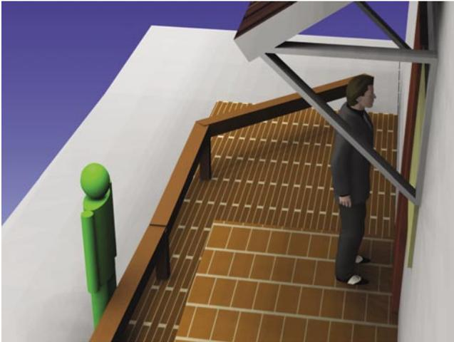
*The same model predicts the view of a camera with 12mm lens mounted in the top right corner. Coverage and %R are clear.*
