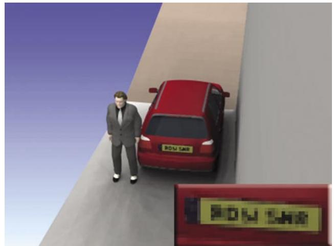
*A supplier says that their proposal will identify vehicles. With this distance & lens a 288x384 pixel image is computed (DVR or VHS playback). The number plate is magnified in the bottom right (inset)*
