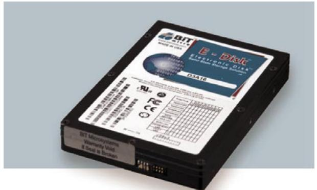
Solid State disks (SSD) are devices that use exclusively semiconductor memory components to store digital data. The memory components are the same ones used for the different types of computer memory: work memory, cache memory and embedded memory.
