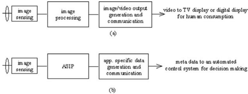
Figure 1: Differences between a normal camera (a) and a smart camera (b).
