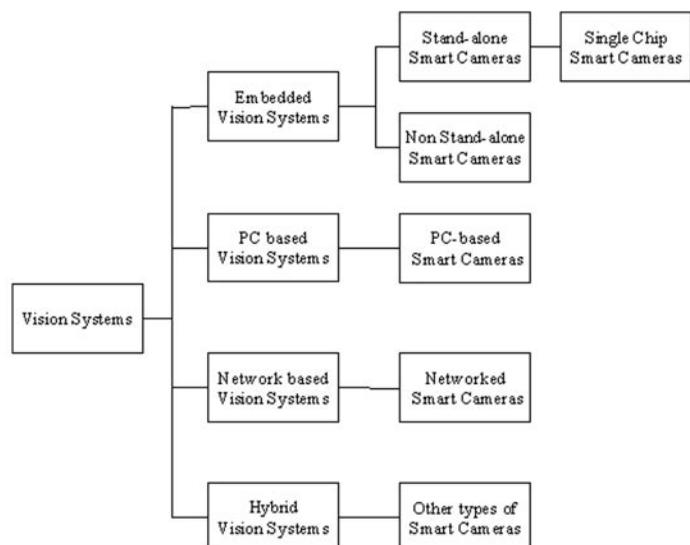
Figure 2: One proposed classification of vision systems and smart cameras.
