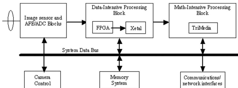
Figure 3: A stand-alone smart camera system architecture for face recognition
