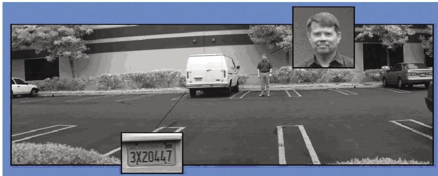
*Figure 4 – SentryScope provides monitoring of large areas with ultra-high resolution zooms of small regions*
