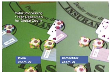
In a high dynamic range scene CCD-based cameras lose important details. With a bright lamp, the table is washed out in a CCD-based camera, but the camera with the D2000 video imaging system gets the details in the table and on the colour chart.
