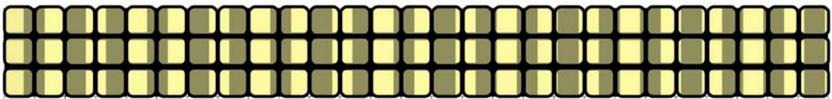
Misalignment of the test pattern projection and the CCD pixels
