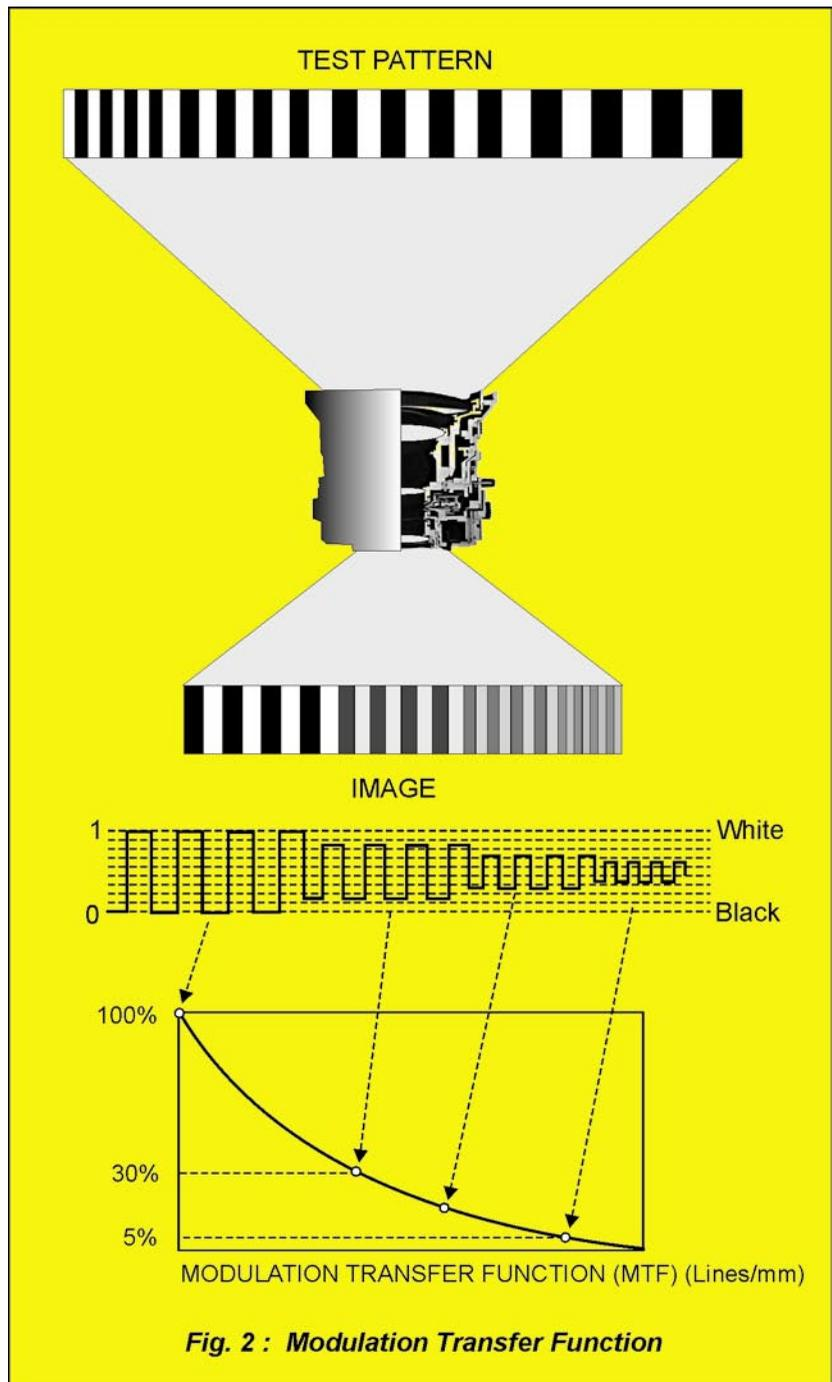
**Fig. 2 : Modulation Transfer Function**
