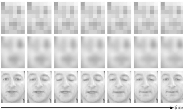
Figure 1: Given only a low-resolution video (top), how can one estimate (or “hallucinate”) the original high-resolution video (bottom)? Unfortunately, simple methods such as bicubic interpolation are insufficient (middle). In this paper we explore zooming using a database of videos with an inference procedure that enforces spatio-temporal consistency of the resulting hallucinated video.
