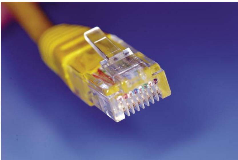
If using Cat-5 as a backbone cable, the additional pairs can be used to power the remote Viva and/or to supply power to the camera.
