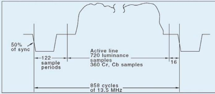
Fig 11 The sample numbering of digital component.
