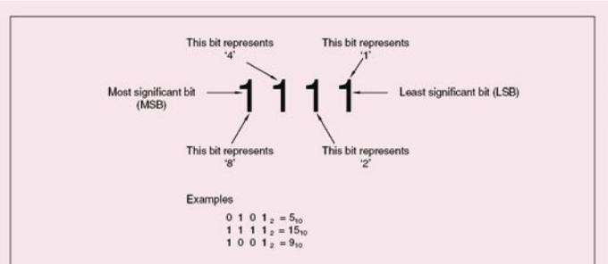
**Fig 2.** A binary conversion table allows any ordinary decimal number to be stored or transmitted by any system which can exist in two states.
