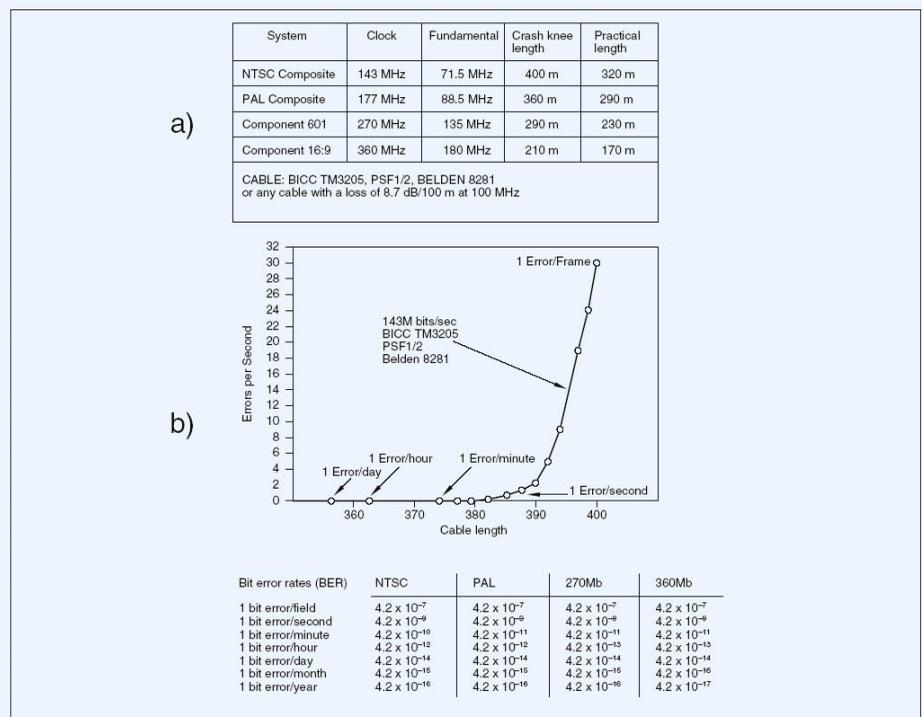
Fig 14 a) the cable lengths which can be used with SDI. Don't exceed them. b) the error rate of SDI rises dramatically at the crash knee. Practical systems must stay to the left of the knee to avoid flaky symptoms.
