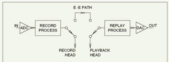
Fig 6 In a simple DVTR with effective error correction, the picture quality in playback is the same as in E-E.
