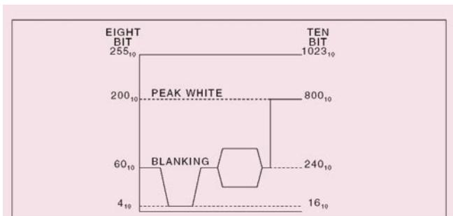
**Fig 10** How the NTSC waveform fits into the eight- and ten-bit quantizing range.
