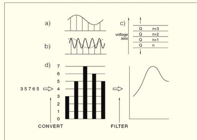
Fig 7 a) A high sampling rate is intuitively adequate, but if the sampling rate is too low, aliasing occurs as shown in b). c) Quantizing divides the voltage range up into equal intervals  $Q$ . The quantized value is the number of the interval in which the input voltage falls. d) Numbers are converted back to voltage pulses, and these are filtered to produce a continuous signal.
