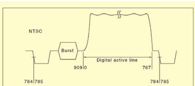
**Fig 9** The sample numbering of digital NTSC.
