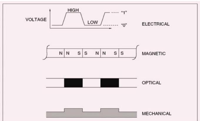
**Fig 3** Several ways of handling binary data are shown here. In electronic circuits, two different voltages are needed, commonly achieved with a simple on/off switch. In magnetic recording, two flux directions are used. Optical recording may use alternating opaque or dark areas and mechanical storage may use raised or depressed areas on a surface.
