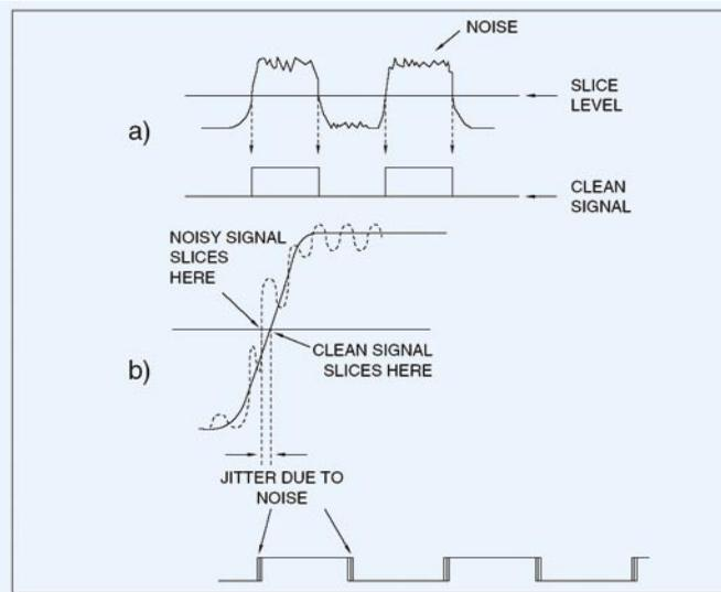
Fig 4 A binary signal has the advantage that a simple slicer shown at a) can be used to recreate a square signal. The result is that noise only causes jitter as shown in b). This can be removed with a phase locked loop.
