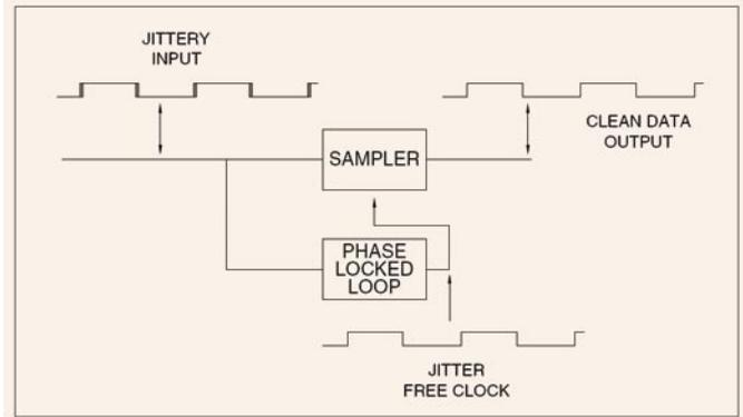
Fig 5 A reclocker uses a phase locked loop to recreate a clean clock which samples the input once per bit and produces a jitter free output. Any number of slicers and reclockers can be cascaded without quality loss.
