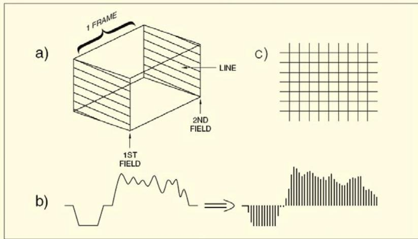
**Fig 1a** In analog television, time is sampled into fields, and each field is sampled vertically to make lines. If each line is also sampled, as in b), an array of pixels will be formed. Such an array can be made from a conventional analog television signal by sampling it a line at a time as shown in c).
