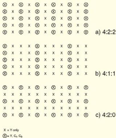
Fig 12 a) Post production standard 4:2:2 sampling in two dimensions. b) 4:1:1 sampling cuts the horizontal colour bandwidth. c) 4:2:0 sampling matches horizontal and vertical spacing.
