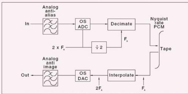
**Fig 8** In an oversampling converter the sampling rate is temporarily increased to ease the problems of filtering in the analog domain. The sampling rate is changed up or down in the digital domain where filtering is easier.
