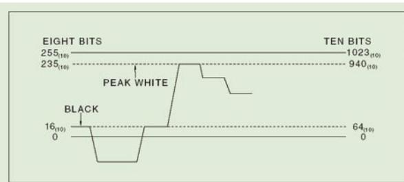
Fig 13 How component video fits into the quantizing range for eight- and ten-bit sampling.
