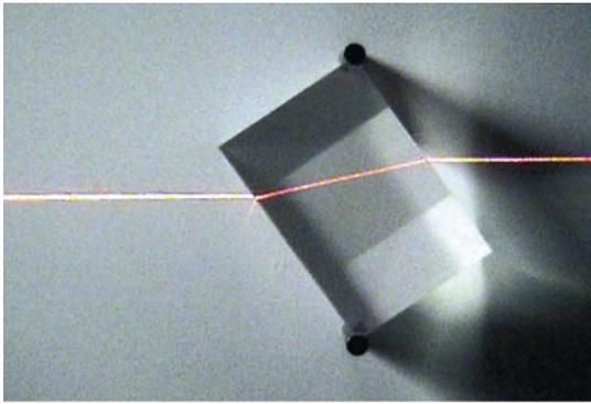
**Laser light refraction through a prism**
