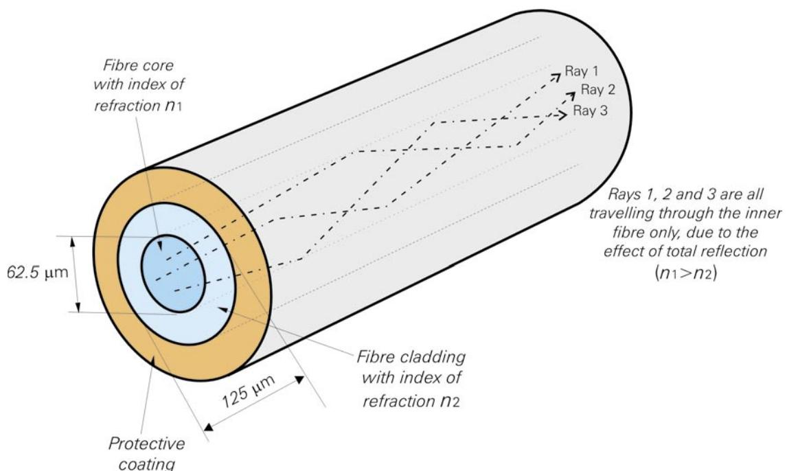
**Fibre optics usage is based on the effect of total reflection**
