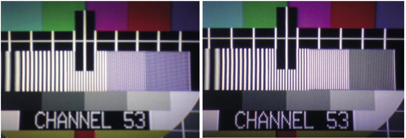
*Photo illustration of the difference between a composite (on the left) and Y/C (on the right) video signal of the same test channel*
