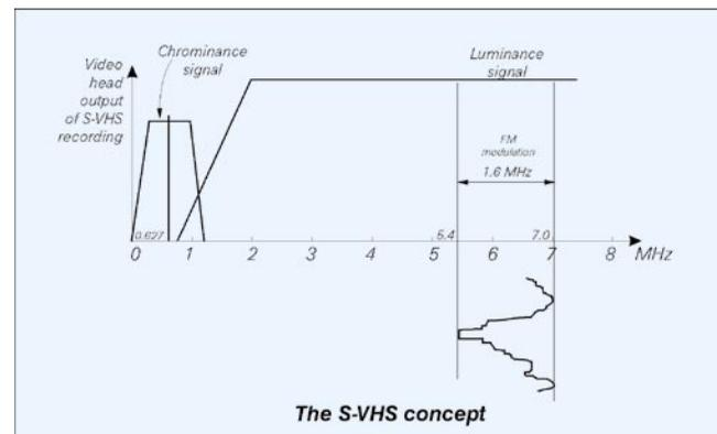
cross-luminance artifacts (see the test images illustration on page 37). In order to minimize such deterioration, S-VHS recorders permit direct input and output of the uncombined luminance and chrominance components.
