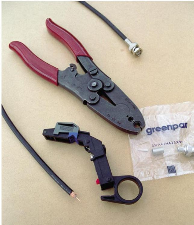
impedance, i.e., RG-59/U is  $75\Omega$ , compared to RG-58/U which is  $50\Omega$ . Next, RG-59/U is slightly thicker, both in the center core and the shield. There are BNC connectors for the RG-58/U which look identical externally, but they are thinner on the inside.
