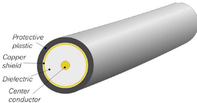
**Cross section of a coaxial cable**
