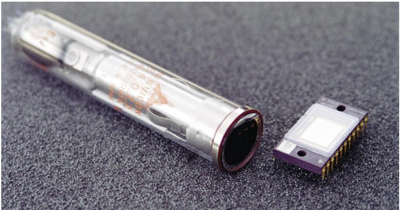
transfer of all the mobile electric charge stored within a semiconductor storage element to a similar, adjacent storage element by the external manipulation of voltages. The quantity of the stored charge in this mobile packet can vary widely, depending on the applied voltage and on the capacitance of the storage element. The amount of electric charge in each packet can represent information.”
